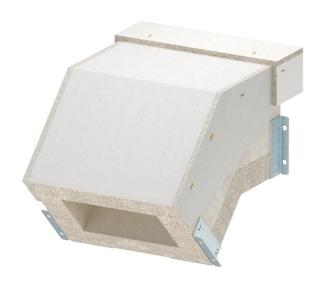
Vertical bend, falling, for PYROLINE® Con S EI90 fire protection duct, type PLCS D091220, consisting of fibreglass light concrete which is resistant to water and frost for the creation of vertical changes of direction (45°) in the duct. Mounted connectors ensure quick mounting in situ, whilst loosely placed covers ensure quick inspection and reassignment.
