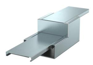
Reducer with intumescent fire protection mesh for symmetrical reduction of straight duct sections from PLM D 0810 to PLM D 0410. Suitable for direct wall and ceiling mounting, mounting below system floors and on support systems. Tool-free joint mounting with PLM SI joint connector. The cover is snapped on without tools, allowing rapid inspection and retroassignment. The cover overhang allows offset cover mounting for continuous equipotential bonding of the entire duct section.
